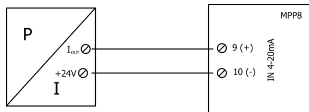
Fig . 21. Example connection of a pressure sensor with a MPP ® 8 series converter equipped with current input A (active)
